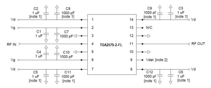
Note 1: Remove cap for pulsed drain operation Note 2: No external load resistor or capacitor is required
